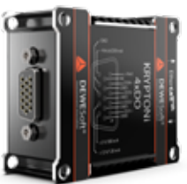
The KRYPTON 4xDO module provides four high speed digital output lines
