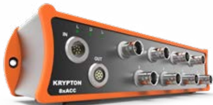
The KRYPTON-ACC is a 4 or 8 channel isolated module for IEPE sensors. Use the KRYPTON-STG with DSI-CHGx adapters to handle CHARGE sensors. Voltage and STG modules can be used with most CAPACITIVE acceleometers.
