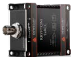
The KRYPTON-1xACC is a single channel isolated input module that handles virtually any IEPE sensor, providing selectable 4 or 8 mA of constant current sensor supply.
