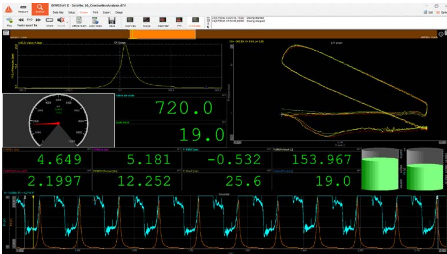
DewesoftX combustion analyzer plug-in, including real-time PV (cylinder pressure/volume) graph
