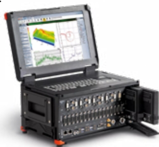
SIRIUS R2DB with built-in, hot-swappable batteries
