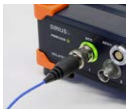
Above: SIRIUS ACC input module, ideal for all kinds of IEPE sensors. The green light around the bezel indicates that the sensor is connected and working fine. Note that ACC+ inputs also include a synchronized SuperCounter® / digital input
